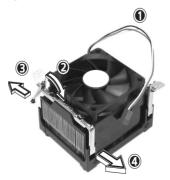
3 Gently push the socket lever down to release the lever and then pull it up.
